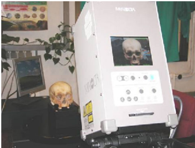
Fig. 4 Acquisition of a skull 3D partial view by the use of the Konica-Minolta laser range scanner of the Physical Anthropology Laboratory at the University of Granada
