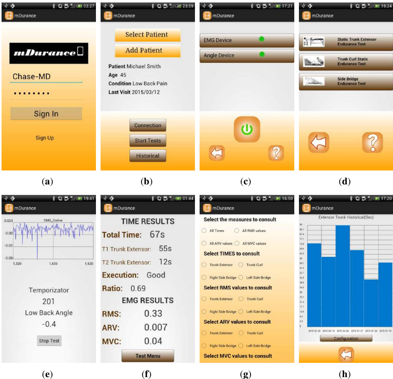
Figure 3. mDurance application snapshots: (a) Login; (b) Patient selection; (c) Sensor connection; (d) Endurance test selection; (e) Test execution; (f) Test results summary; (g) Selection of historical attributes to be represented (part of); and (h) Historical representation.
